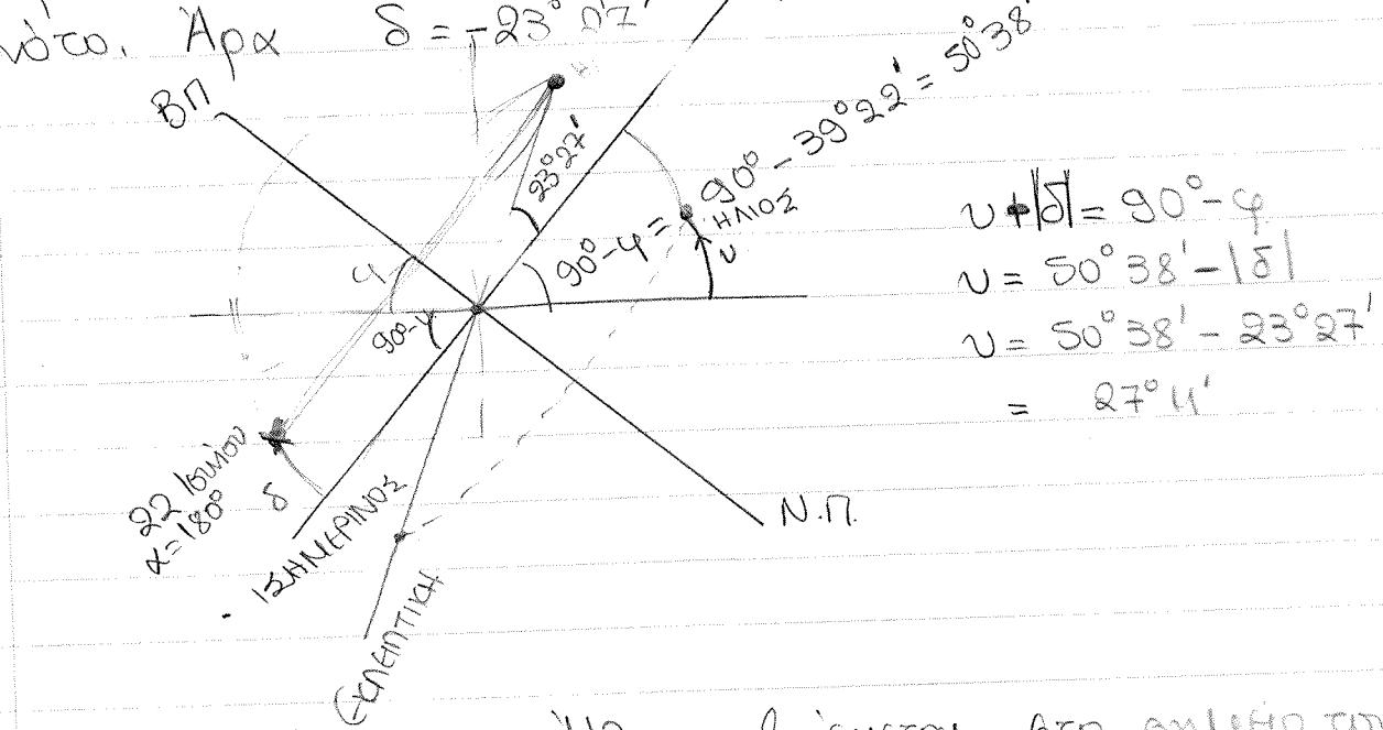
$$\begin{aligned} \nu + |\delta| &= 90^{\circ} - \varphi \\ \nu &= 50^{\circ} 38' - 15^{\circ} \\ \nu &= 50^{\circ} 38' - 23^{\circ} 27' \\ &= 27^{\circ} 11' \end{aligned}$$
