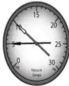
Leaking Intake Manifold Steady Low 5-10 "hg
