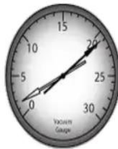
Clogged Exhaust Needle Drops While Accelerating
