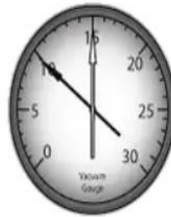
Check Valve Timing Steady Low 10-15 "hg
