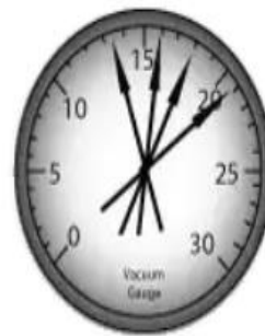
Sticking Valve or Misfire Fluctuating Needle
