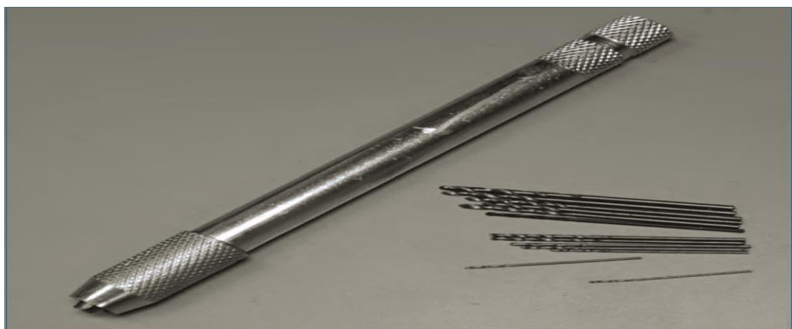
Figure 7: Pin assurance check using the smooth shank of a welding tip cleaner or a micro drill bit could also be used if you don't have a correct diameter terminal test probe. These items are inexpensive.
